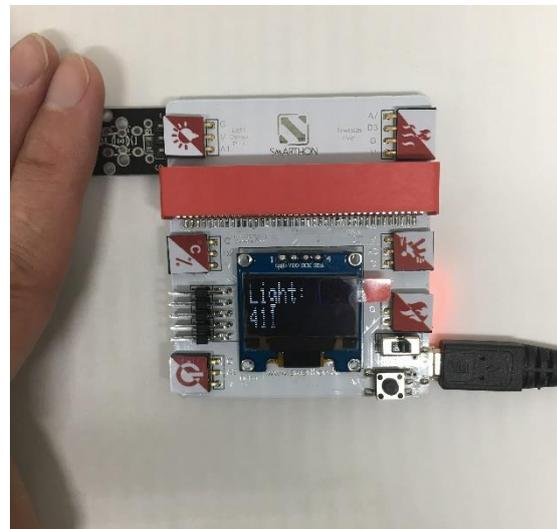
When there is a light turning on, the light sensor value is around 280-300; otherwise when you use a finger to cover the light sensor, it has increased into around 450-470. It reveals that the ambient lighting are getting brighter, the number of the light sensor value shown on the screen is getting smaller and vice versa.
