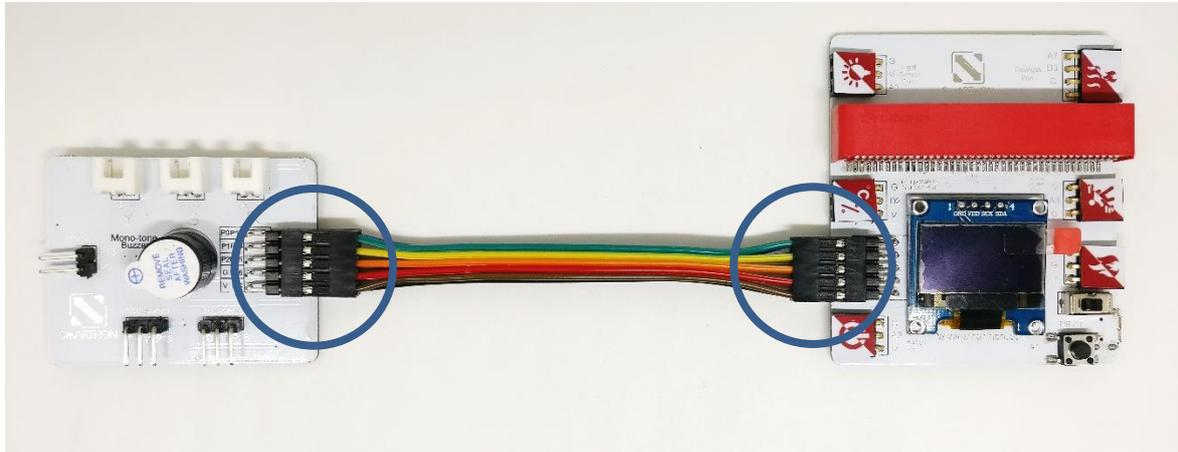
\*To make sure the connecting wire is on the same direction.
