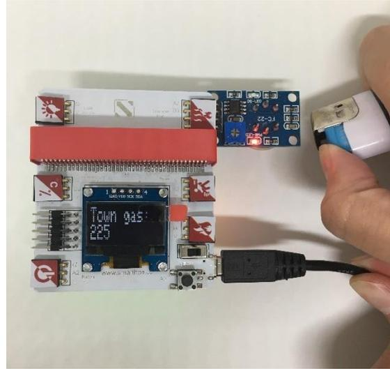
In the normal condition, the town gas sensor value is around 30-50; while there is a town gas leakage, the number has increased from 200 – 850 subject to the concentration of different leakage velocities.
