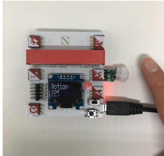
If this sensor detects any movements, the value of the motion sensor will increase from 0 to 200, as shown in the picture.
