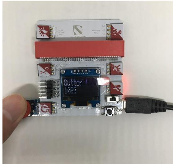
When you plug in the button, the screen shows 0 or 1 (small number); while when you pressed the button, the screen shows around 1020 - 1023 (large number). It indicates that a large number will be shown when you pressed the button.
